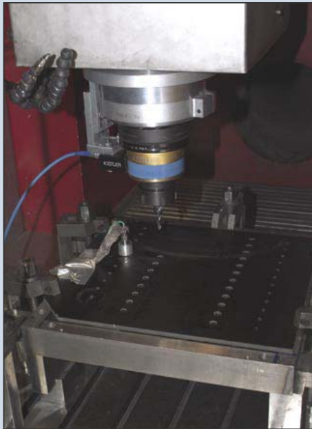
CFRP platter is machined with a diamond coated countersink drill.
