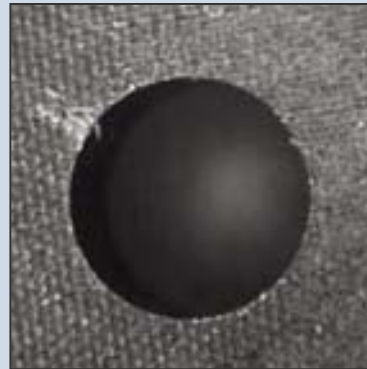
The result with an optimized drill is a clean drilling hole without CFRP delamination.
