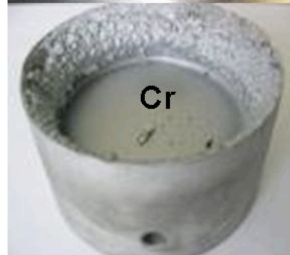
S63N 2500Ah end of lifetime occurring tunnel effect 穿隧现象
