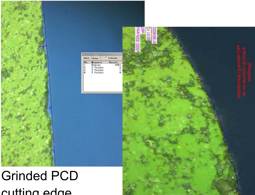
Laser processed PCD cutting edge
